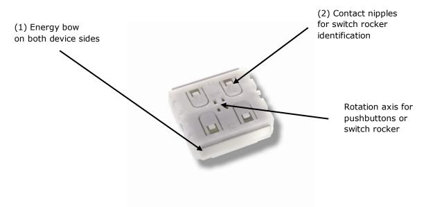
Electro-dynamic powered radio transmitter device PTM 21x
